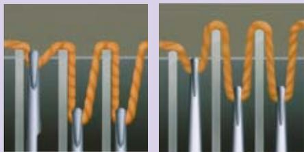
Conventional latch needles offset in grooves      Slide needles centered in grooves
